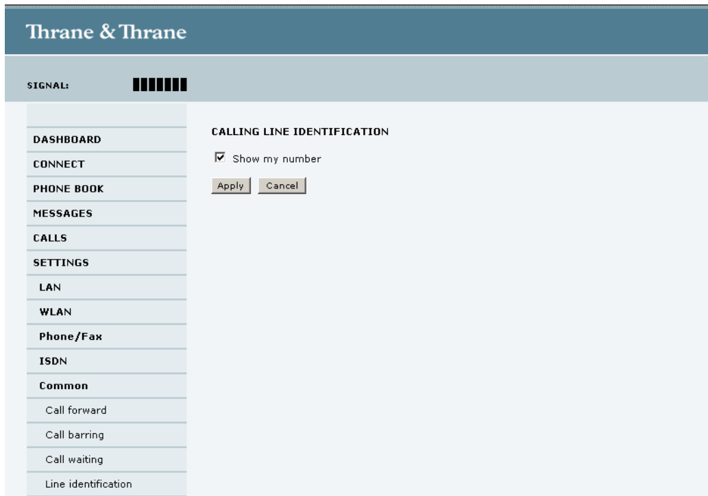
Figure 6-30: Web interface: Settings, Common, Line identification
